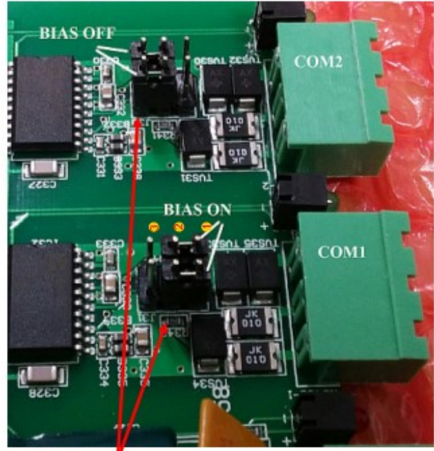
Board and orientation of the RS485 Bias resistor jumpers:
